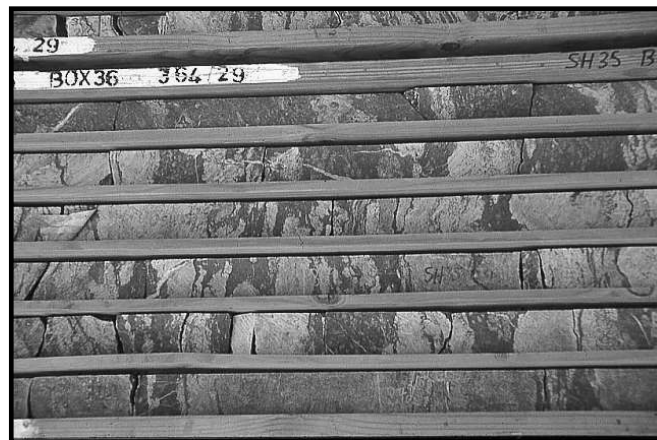
Figure 1: Chromititic Peridotite - the black material is fine-grained chromite and the light grey is altered talcose peridotite
