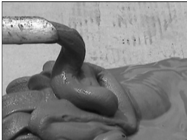
Figure 9. Correct consistency for a pumped grout
